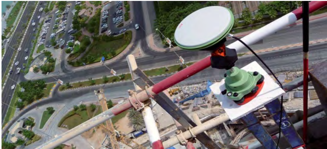
Figure 6: LEICA GNSS System for precise Survey
