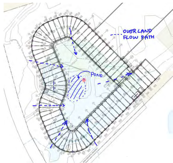
Figure 2: Structure and overland flooding path
