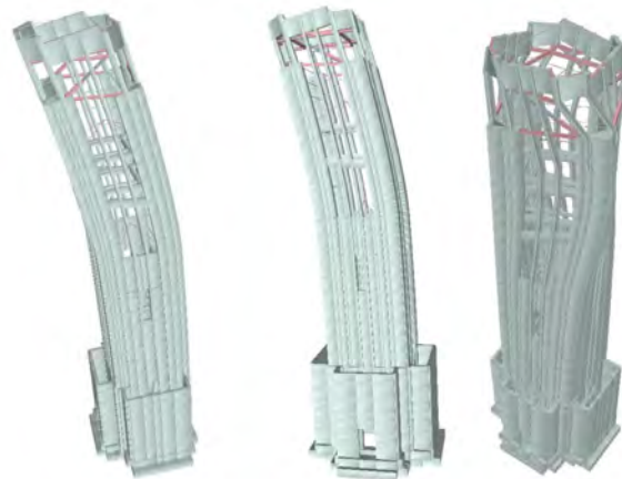
Figure 4: Fundamental modes of 0.85s X translation, 0.81s Z translation and 0.13s torsional translation (strengthened building).
