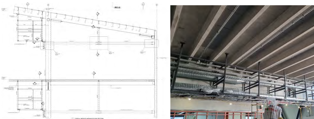
Figure 4: Section through F&P “Shed” and photograph of the services highway
